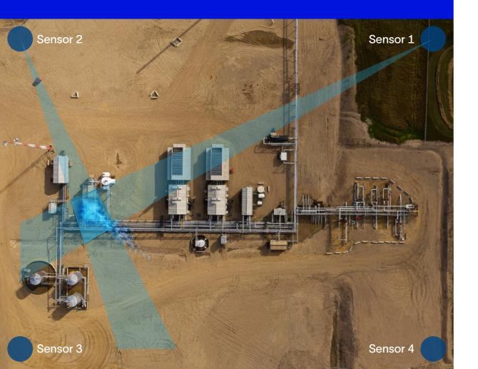
The OGMP 2.0 pathway takes you through five levels of measurement and reporting methane emissions. The Gold Standard requires both source-level and site-level measurements. SEES provides all the technologies needed.
