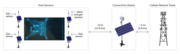
The methane point instrument delivers a continuous methane emissions monitoring system consisting of connectivity stations positioned up to 3 mi [4.8 km] from the nearest cellular network tower. These stations can communicate with as many as 200 sensors or locations within an 8-mi [12.9-km] radius.
